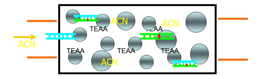
The heteroduplexes with mismatched basepairs at the point of mutation elute off the cartridge first
